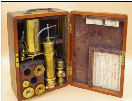
Hopkinson patent swivel-arm non-amplifying indicator serial #217 built to a patent of 1869. Of the some 1200 believed built, only seven of these indicators are confirmed in existence today world-wide, and this example (cased with its complete set of accessories including a whalebone ruler) resides in the writer's collection. Photo by Peter Evans.
