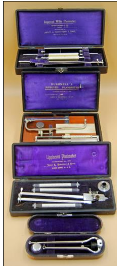
A selection of American planimeters from the writer's collection. These were used to measure the area of an indicator diagram as the first step in determining the mean effective pressure in the cylinder.
