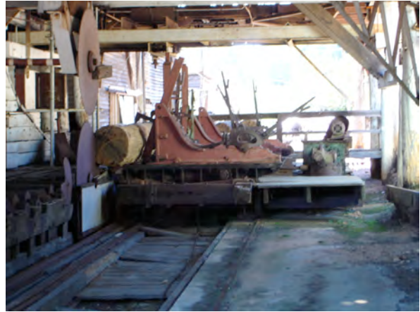
Donnelly River sawmill, log carriage and twin breaking down saws. Photo: John Dargavel
