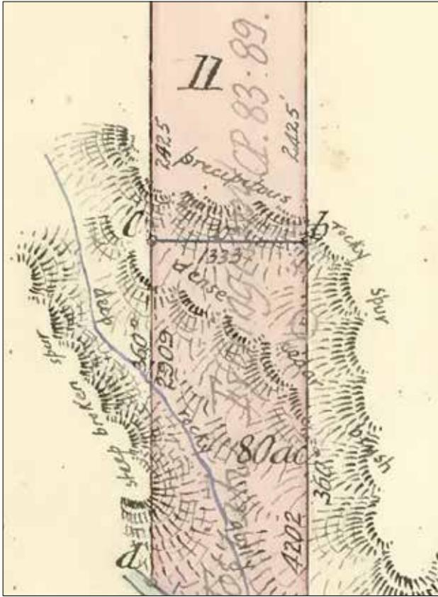
**Figure 6:** Enlargement of part of the plan of Portion 11, Parish of Albert, clearly shows the surveyor's annotation 'dense cedar brush'.
